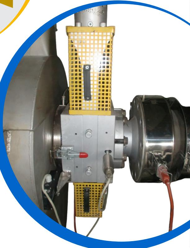
Equipped with an integrated pressure transducer, the HSSC automatically initiates the screen change when the system reaches a predefined pressure. A visual signal lamp indicates the ongoing change process.
