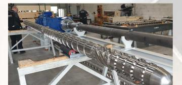
GTS offers high quality single screws with all types of mixing, Maddock and barrier zones for all polymers and applications. Cascade extrusion, multiple venting and a large number of applications and designs for recycling processes are our daily business.
